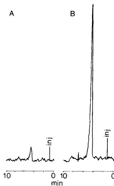
Figure 1 Supercritical fluid chromatography of [ 14 C]propranolol, with in-line radioactivity detection on an amino-bonded column with supercritical carbon dioxide and methanol (90:10) containing 0.1% triethylamine at 50°C and 5 ml min -1 ; (A) 10,000 dpm and (B) 100,000 dpm on-column.
